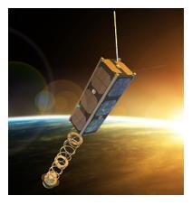
**D-Star One** is a <u>3U CubeSat</u> designed and built by German Orbital Systems as a technology demonstration for their planned CubeSat communications constellation.
