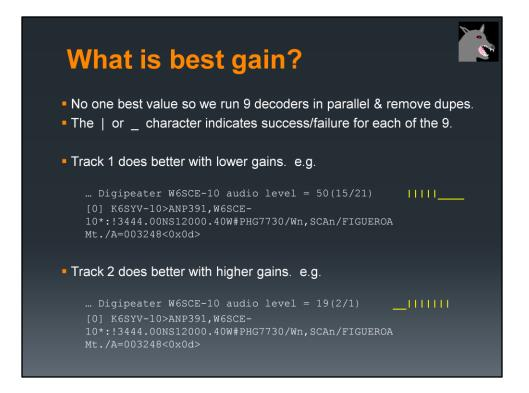
On the right side we have an indication of which decoders were successful. The vertical bar means an error free frame was received. An underscore means failure.
